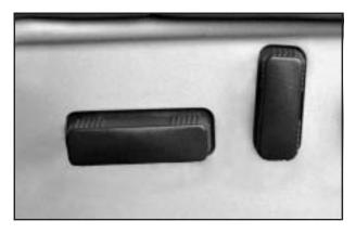
If your vehicle has power seat(s), the controls are located on the outboard edge of the front seats.
